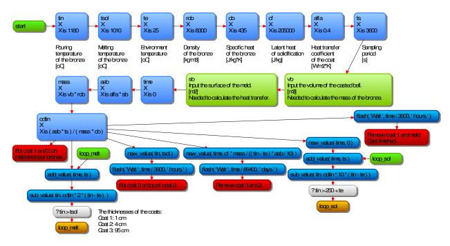
Fig. 5. The Visirule implementation of the control algorithm
