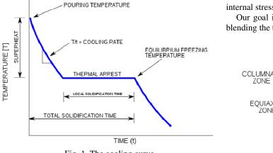
Fig. 1. The cooling curve
