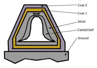
Fig. 4. The complete coating of the cooling mold
